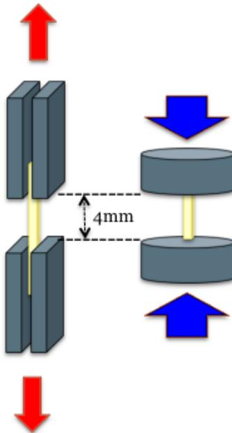
**Figure 2:** Diagram showing the setup of the Instron machine. The specimen was first placed inside the instron which pulled the sample, applying tensile forces. As the material is being pulled, its elongation could be automatically observed and documented by the Instron machine. Over time this will output a resulting curve or tensile profile showing how the materials react to the forces being applied. The sample was cut and repeated in compression.
