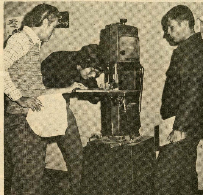
BAND SAW OPERATION -Jack Bolin, left, instructs Bill Landers on sighting in, while wearing safety goggles, and adjusting band saw used in the initial cutout of plaque designs. Lonnie Griffin, right, observes procedure while awaiting his turn to operate the machine.
