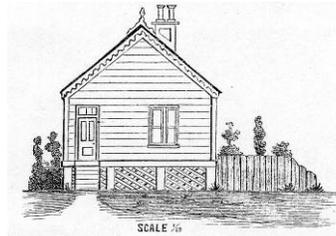
may be dispensed with, and the space now given to the stairway and dressing room be equally divided into two rooms, measuring each 8' x 10'. By a sufficient elevation of the roof two very serviceable apartments may be made in the garret. Of course the cost of this building may be very much increased by elaborate external or internal finish. The estimate above given includes painting and plastering, and supposes all the workmanship to be in a neat but simple style.
