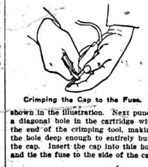
shows in the illustration. Next punch a diagonal hole in the cartridge with the end of the crimping tool, making the hole deep enough to entirely bury the cap. Insert the cap into this hole and tie the fuse to the side of the cartridge.
